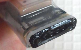
The paint shall be tried in about 1 hour. It is recommended to apply a second paint layer for easier removal of the paint. If the paint layer is too thin it may get difficult to remove it in one piece. Once the paint is dry, the device is ready to get deployed.
