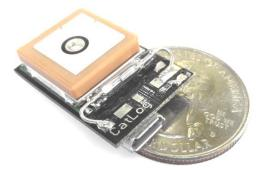
Used in thousands of GPS tags around the world CatLog became the standard GPS data recorder for wildlife bio-tagging. The device will record the position in an adjustable time interval. The movement profile can later be displayed on a map or exported to use with other software.
