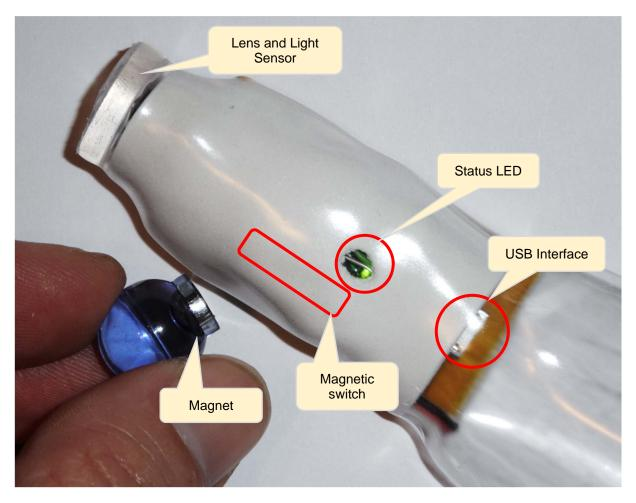
The camera can get modified for battery size, lens tilt angle, solar charging. These options need to get adjusted to your requirements and embedded during production. Please get in contact with our engineering department (engineering @ perthold. de).
