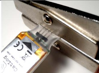
Now quickly take the device, place the seal area between the jaws (center area) and close the clamp. It is important to note to **not clamp parts of the device**.
