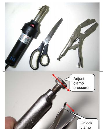
The ThermoSeal material is handled like regular shrink tubing. You will need the following tools: Heat gun, seal clamp and scissors.
