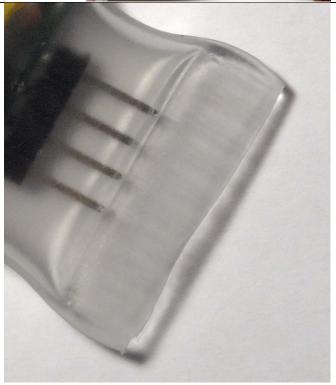
After about 30-60s you can unlock the clamp and remove the device. In batch operation you will heat the next device while the seal of the previous device cools down. Please remember to let the clamp cool down itself from time to time.
