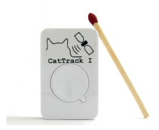
The device is water resistant, has an internal rechargeable battery which allows extended usage of 30 hours and more. The interface for recharging and data transfer is USB. The position capture interval time can be adjusted by the user. Captured position data is displayed directly on Google Maps (Internet required).
