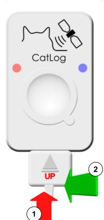
1: Plug in the connector into the CatLog. The arrow on the connector **must point upwards**.
