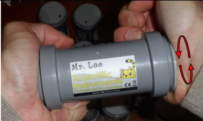
**Important:** In some cases it is not sufficient to just press the cap into the tube. The gasket may not engage properly. It is advised to hold the enclosure between the palms of your hands and rotate the cap as shown in the picture. On a proper engaged gasket you will not be able to remove the cap by hand.
