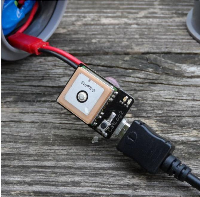
GPS can now get accessed and connected to USB communication cable (note: for communication a special cable is required)
