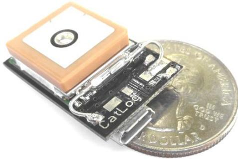
Used in thousands of GPS tags around the world CatLog became the standard GPS data recorder for wildlife bio-tagging.
