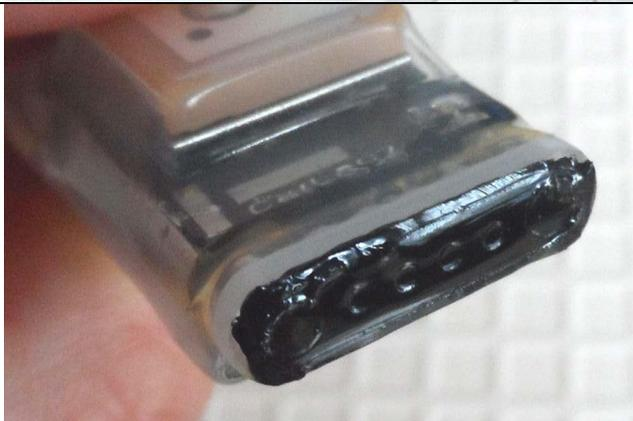
The paint shall be tried in about 1 hour. It is recommended to apply a second paint layer for easier removal of the paint. If the paint layer is too thin it may get difficult to remove it in one piece. Once the paint is dry, the device is ready to get deployed.
