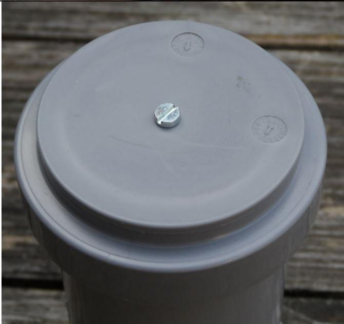
Place screw into purge opening, drive screw in until screw head touches plastic surface, do not over-tighten it (skip if cap has no hole).
