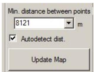
The value of minimum distance tells the program that all points with a distance lower than the defined value will be filtered out. The value can be selected manually or automatically based on the map scale. Button “Update Map” needs to be pressed each time the value was changed manually or the map was zoomed in/out.
