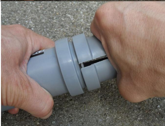
Put your fist around the tool and slightly pull in lateral direction to lose the cap a bit to get more grip with the tool clamps.
