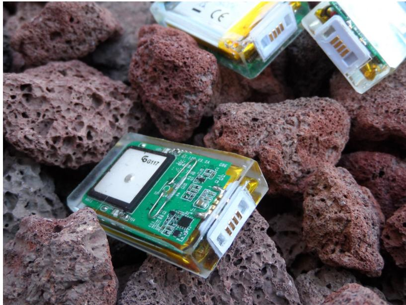
Other than devices in ThermoSeal, which are hermetically sealed, Potted devices have their interface exposed to the environment. This requires a different type of connector.
