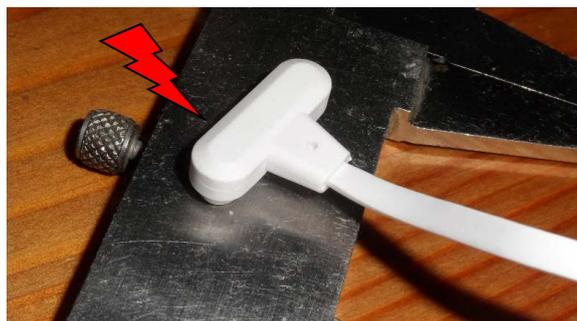
Since the contacts need to stay clean to allow good connection, but the devices are used in the field there is a solution for this contradicting situation. For devices which are deployed with exposed interface we supply a so called peel-off protective paint. The procedure to apply and remove this paint is explained below.
