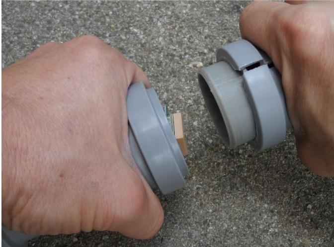
Firmly pull the tool in a straight line from the enclosure. It will pull out the cap.
