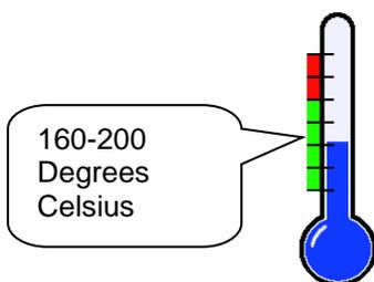
Next step is to adjust the heatgun. The optimal temperature range is 160-200 degrees Celsius (320 – 390 Fahrenheit). If you have an unregulated heatgun you will need to vary the distance between air outlet and device to not overheat the material. You may also want to shield the battery. The battery may get damaged by too high temperatures.
