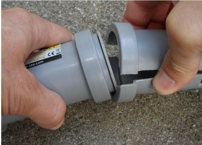
First, locate the cap with the larger diameter, it will cover the GPS unit.
