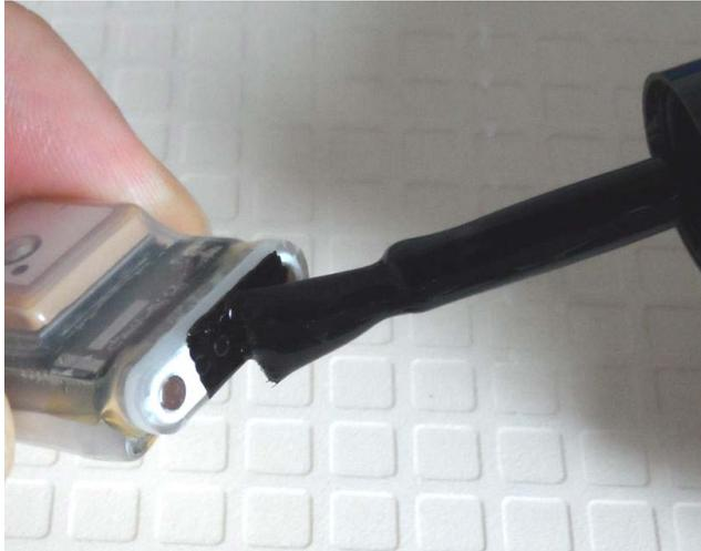
Shake bottle well before use. Take small brush and apply a layer of paint over the connector.
