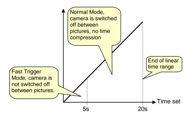
With firmware version 2.2 a **Time Compression** feature is implemented. This makes the adjustment of longer interval times more convenient.
