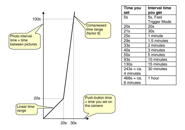
An application hint for the VistaQuest camera for setting the delay time without any hardware additions: For this the On/Off switch of the camera is used. Pin Set Delay is connected to Pin On/Off,
