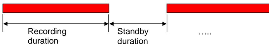
The smallest time increment for these durations is called a time unit. The length of a time unit is specified in the data sheet and can be factory set depending on customer needs. If nothing is specified the standard equivalent of 1 time unit is about 15 minutes.
