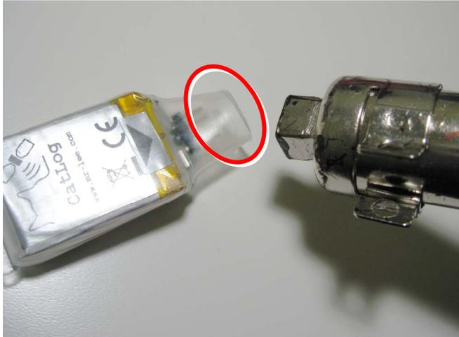
Now heat the material at the sealing location (see red circle in image) from **all sides** until it gets soft and sticky. If you are opening a seal apply heat until the material gets back to the tubular shape. Do not overheat or apply heat for a long period of time. Usually it takes 30s to 1 minute to properly heat the material.
