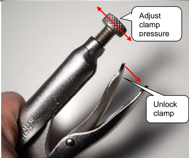
Before you start adjust the sealing clamp. With the adjustment wheel you set the clamp force. Make the adjustments while the clamp is open, when close the clamp to see the resulting gap size/pressure. The clamp will lock itself in closed position making it very convenient for the later sealing operation. To unlock press the handle lever as indicated in the picture below.
