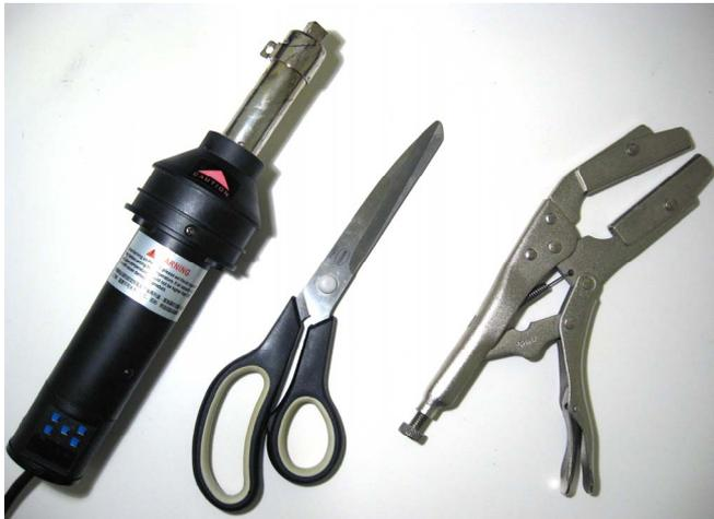
The ThermoSeal material is handled like regular shrink tubing. You will need the following tools: Heat gun, seal clamp and scissors.
